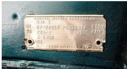
Notice the '67 trim tag and evidence it was tampered with i.e. reinstalled and possible peening over of the left rivet when tapped back into the factory hole. The car screams '66 but the tag says '67
